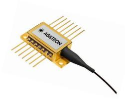
The 785nm series laser diodes are fabricated in a hermetically sealed 14-pin butterfly package. The laser diodes contain a monitor photodiode, thermoelectric cooler (TEC), and a thermistor to secure high-quality laser performance. Our laser products are Telcordia GR-468 qualified and in compliance with RoHS Directives.
